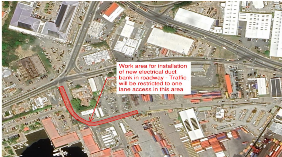
Image: Crown Bay Road work area for the Feeder 9A Underground Electrical Project.
